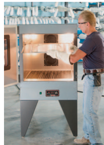
Heating thermoplastic prior to shaping over positive mold.
