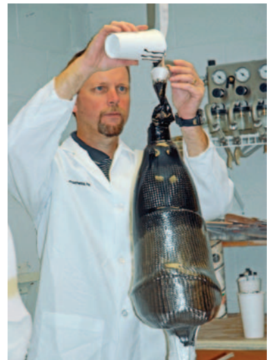
Adding catalyst-pigment mixture to activate socket lamination.
